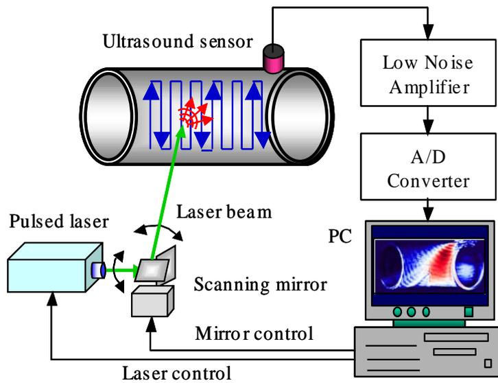
Fig. 1 LUV System Configuration
